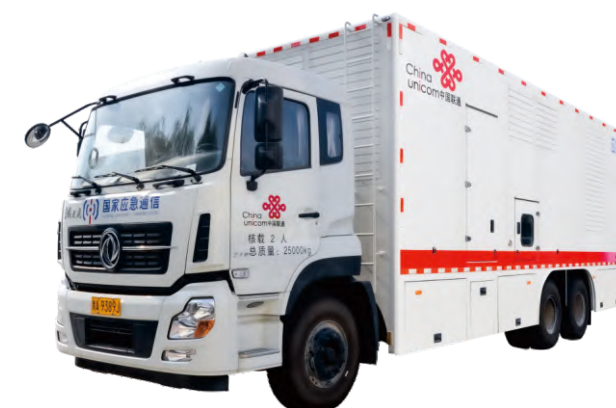
600kW Automobile Power Station
