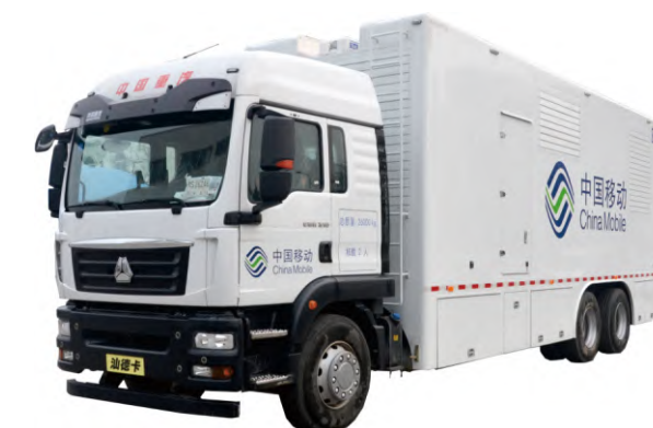
800kW Automobile Power Station
